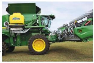
Stauffer unit and Montag. We went with Montag, but our mount could handle either one." Puck explains that they felt the Montag was more horsepower-efficient, and the metering augers were more consistent than Stauffer's venturi style.
